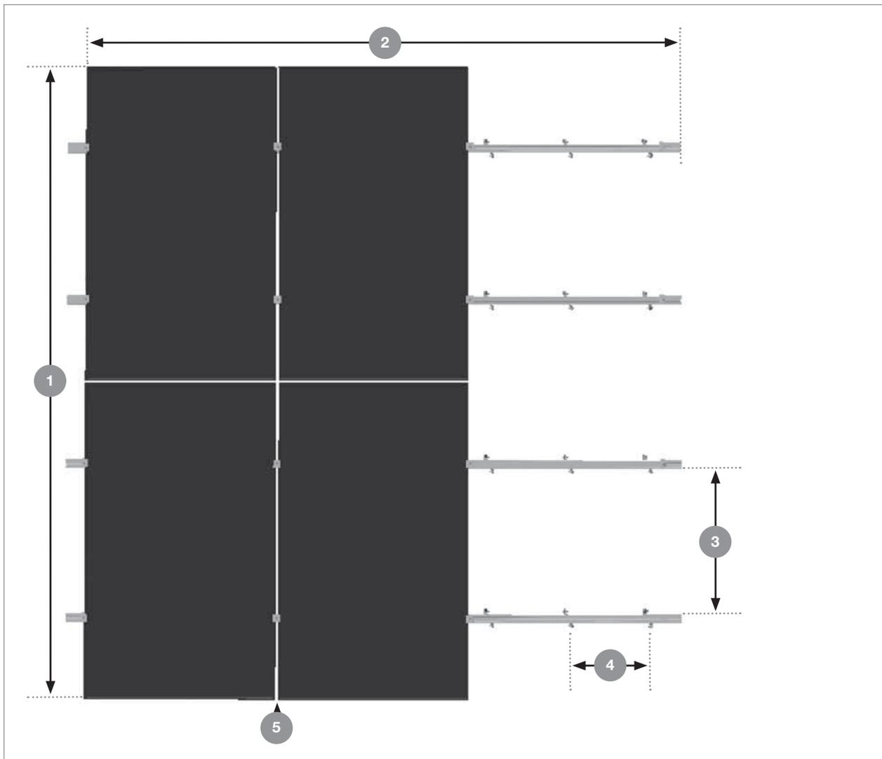
1. Height of the module field: number of modules in the vertical x module height
