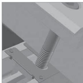
Low-resistance connection between the modules and base rails:
