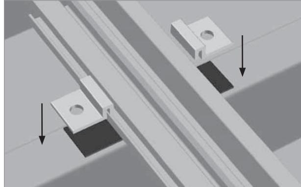
Positioning of the trapezoidal top fixations for bead heights < 20 mm
